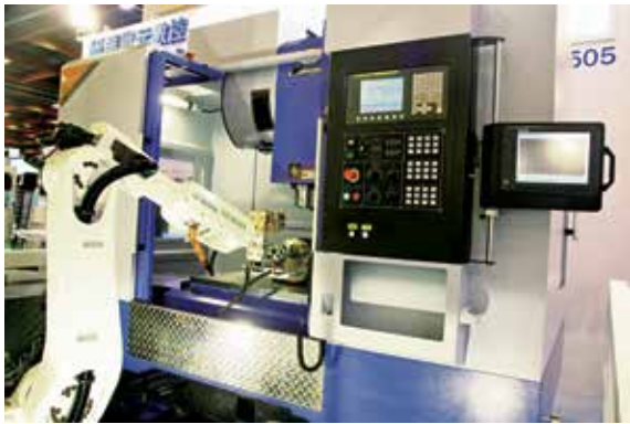
凱柏精機機台加裝IFC整合機械手、分度盤，主軸震動偵測與IP camera
